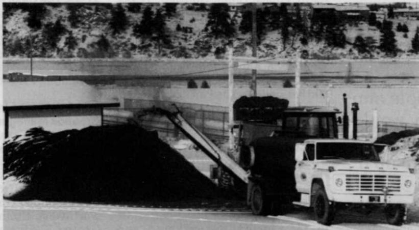
A cone-type grinder is much less expensive to operate than standard tub grinders for making compost. It's also safer and faster.
