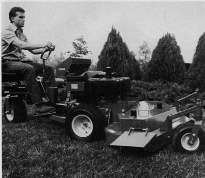
Bunton's BR 61 is an 18 hp rider with an Onan engine.
