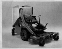
out of the tight spots. The rear discharge to grass collector design allows close trimming on both sides of the mowing deck.
