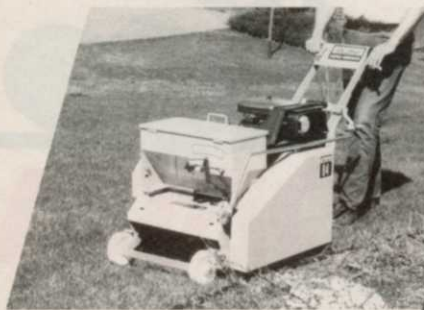
MODEL 84 walk-behind slit seeder, 18 hp, self propelled.
