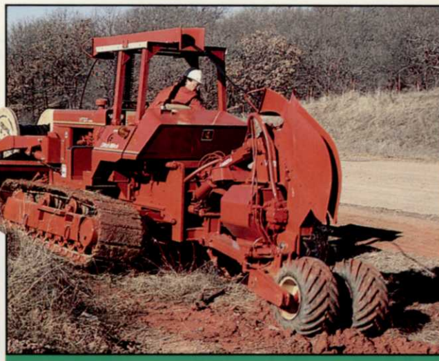
High performance vibratory plowing is possible with the HT100 hydraulic track plow.
