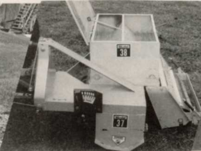
MODEL 37/38 for tractors in 16-25 hp range, bare dirt capabilities with dual feed hopper.
