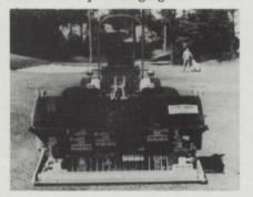
sixteen inches. Tines pivot back and forth, causing a "lifting" effect in the soil, and combines penetration through the soil pan for vertical drainage with the shattering effect of the compacted layers for thorough aeration.
