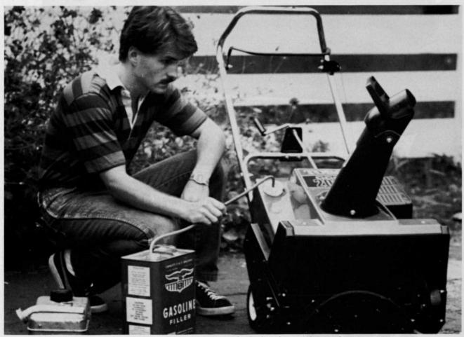
To completely drain your snowthrower of gas, first empty the fuel tank according to the instructions in your operator's manual. Then, start the engine and let it run until it stops.
