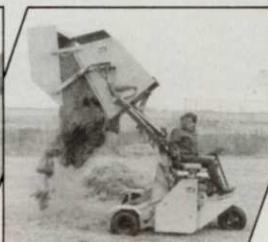
Feel like your grass clippings may be getting ahead of you? Try this model 54HL 5' self-propelled sweeper unit with high lift for large area cleanup. 24hp engine, hydraulic-drive, with optional thatcher, sweeps wet or dry materials using 'sure-grip' rubber fingers.
