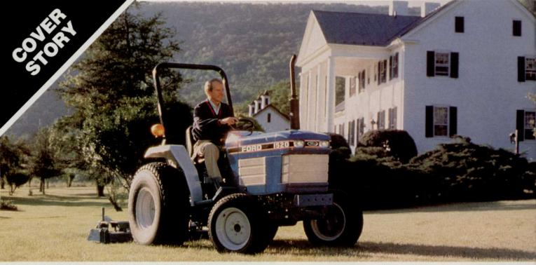
Ford's 1520, at 19.5 hp, is in the middle of the company's compact tractor power range. It can utilize more than 50 implements and attachments.
