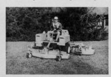
144-inch rotary cut machine, it features hydraulic drive wing decks, direct-drive front deck and hydraulic lift on all decks. The machine folds to 78-inch width for easy transport, with a maximum ground speed of 9 mph. It carries a 20-gallon fuel tank and 20gallon oil tank with oil cooler. The fail-safe hydraulic-release torque
