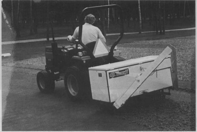
The CoreMaster 12's quadratine design improves aeration pattern efficiency and maintains a 31/2-inch penetration depth with each pattern.
