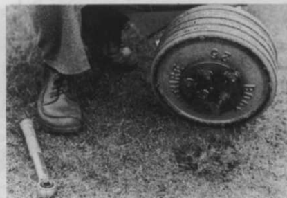
Measuring traction: the force to tear the studs through the grass is measured using a dial-indicating torque wrench.
