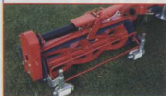
Fixed cutting unit, with anti-scalp rollers.
