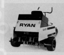
The throttle, choke and ignition switch are also hand-operated while speed, brakes and lift control for the aerating head are controlled by foot pedals. The machine has hydrostatic drive, and transport speed is 6 mph, nearly double that of other aerators.
