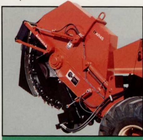
Earth saws are designed to dig in tough conditions, and feature carbide bits that are easy to change.
