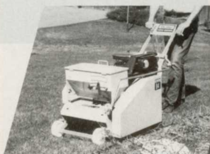
MODEL 84 walk-behind slit seeder, 18 hp, self propelled.
