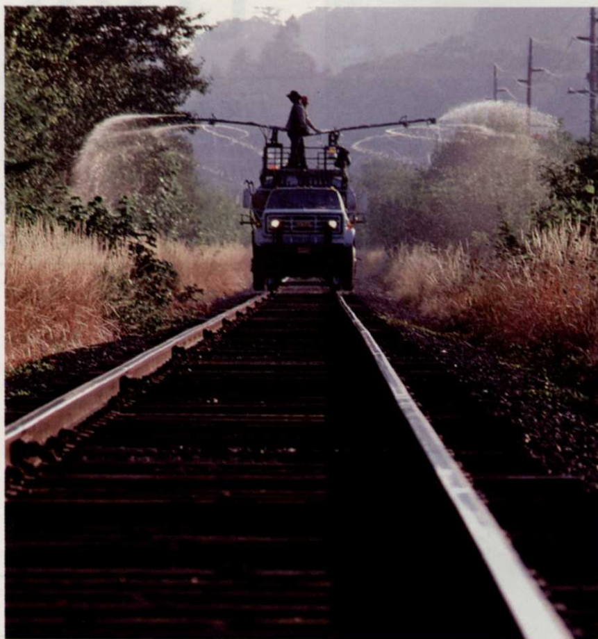
Spraying pesticides from booms mounted on trucks or railroad cars is one of the most efficient ways of controlling rail-side vegetation.
