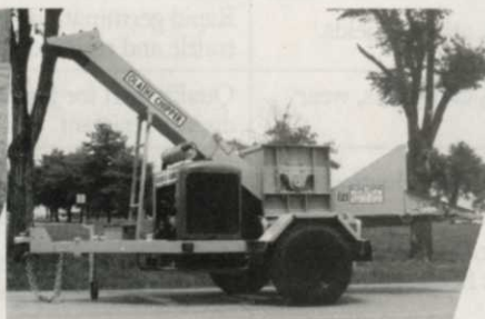
Model 816 — Debris chipper handles kiln dried lumber and assorted wood debris.
