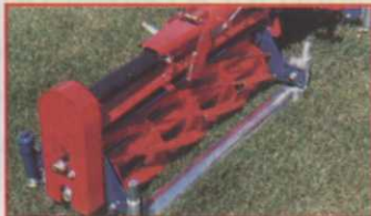
Floating cutting unit with front roller
