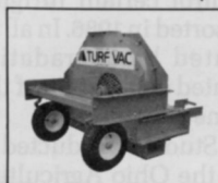
MODEL FMB Front-mounted blower. Easy manual control of left/right/front on-the-go discharge.
