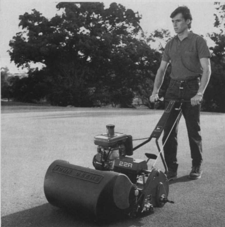
Walk-behind reel mowers, like this John Deere 22R, are used for many golf course greens.
