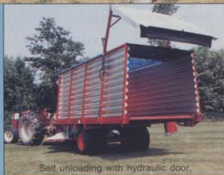
Self unloading with hydraulic door.
