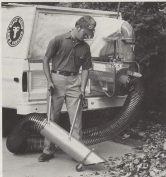
Use the heavy duty wheeled blower to move large quantities of leaves toward the truck.
