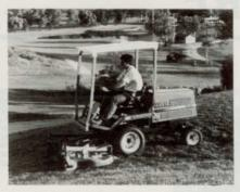
lifted hydraulically, with cutting heights from 1.5 to 4.0 inches. Independent front brakes allow for zero turning radius at mowing point by applying one brake.
