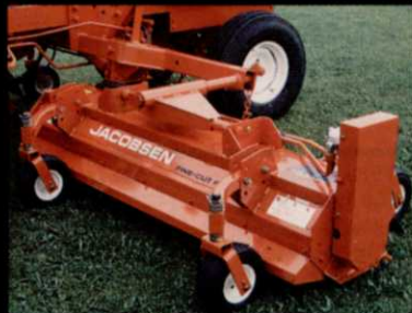
The HR-15 is also available with "fine-cut" flail decks. Jacobsen exclusives for a superb quality cut.
