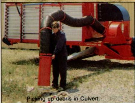
Picking up debris in Culvert.
