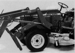
Loaders like this one can be easily removed from tractors in less than one minute. This quick-change features makes the tractor more versatile and time-efficient.
