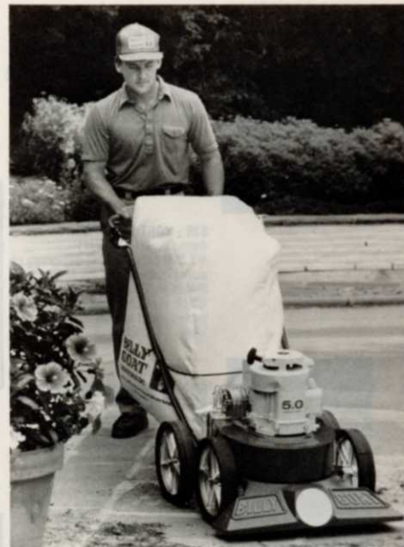
The suction sweeper is used for sweeping up leaves in outlying areas, away from the truck.
