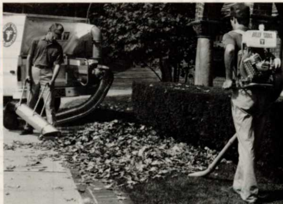
Use the backpack blower to remove debris from shrubs and hard-to-reach areas.
