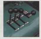
For added convenience, specially engineered hydraulic system allows backlapping of individual reel units while on mounts.
