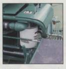
For minimized downtime and increased life of hydraulic components, features 10-micron oil filtration system.
