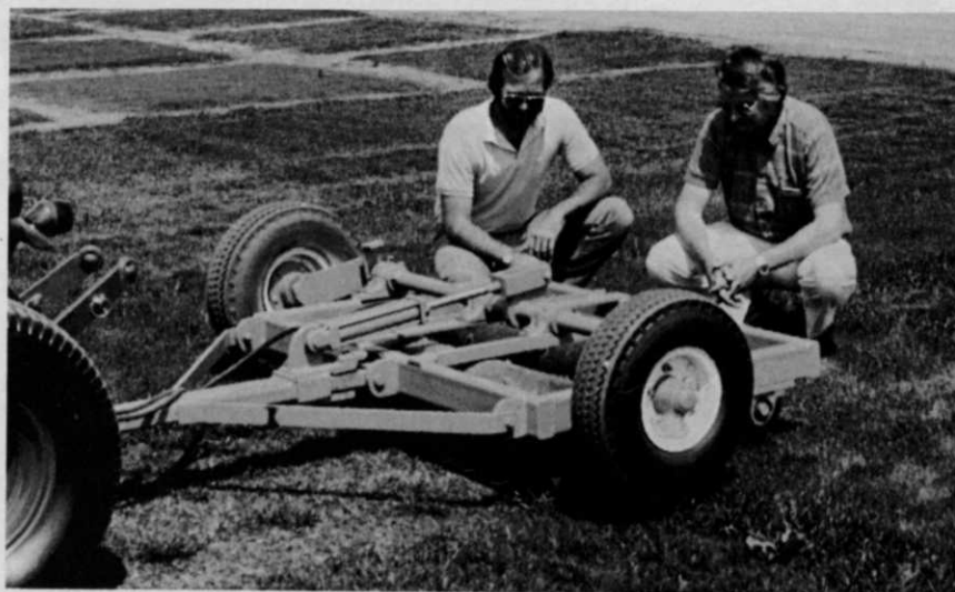
Matt Leonard and Steve Cockerham look over the traffic simulator they created to produce wear on athletic field research plots.
