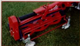
Fixed cutting unit, with anti-scalp rollers.
