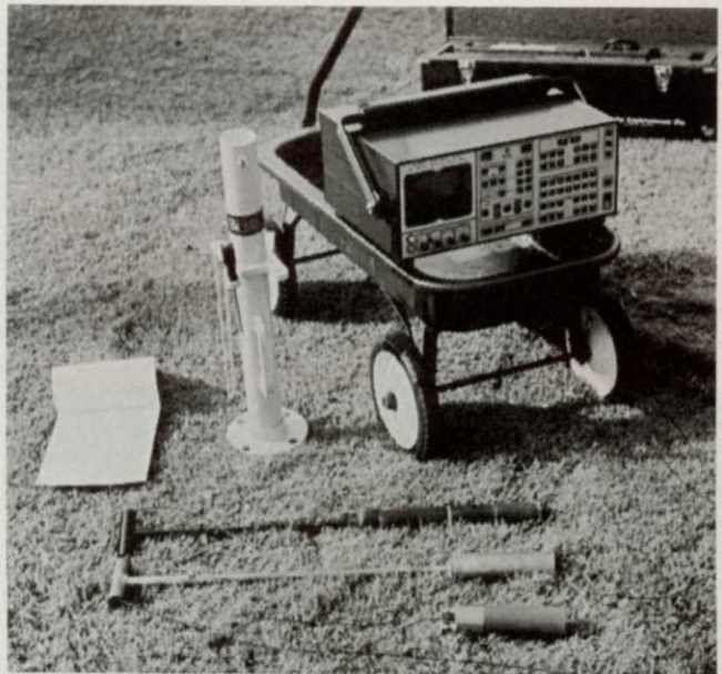
Penn State University uses a Clegg impact tester and vibration analyzer with three different weights for their impact absorption research.
