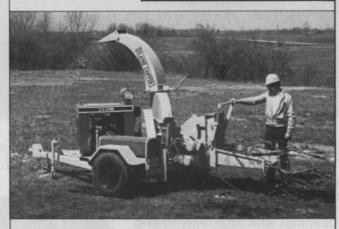
MODEL 986. Compare its 42" diameter drum, hydrostatic drive for variable feed speed, 15° curbside angle for operator safety and 360° swivel chute. Gas or diesel — you'll buy Olathe.
