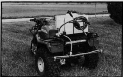
diaphragm pump, a pressure gauge and a heavy-duty toggle switch directly behind the operator's seat.
