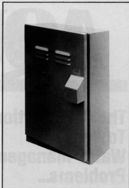
Installation is aided by a new anchor-bolt template which allows the unit to be mounted accurately on a concrete pad without using any additional tools. A 3/4-inch waterproof plywood panel permits the installer to place controllers or other equipment in any desired configuration.
