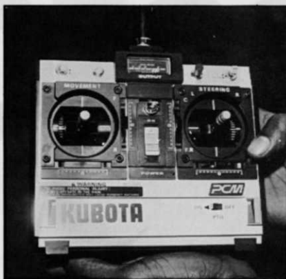
The Kubota PX-2100 control box which controls the tractor up to 300 feet in ideal conditions.
