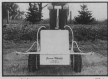
ground-driven pumping system. This new model features larger, easy-topush pneumatic-type rubber tires and
