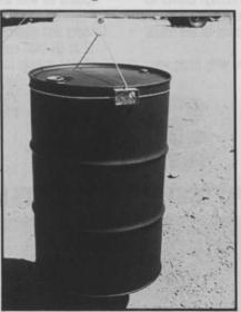
the end to transport them has been designed by Free Enterprise Systems. The Bold Eagle Barrel Harness can lift any 55-gal. or smaller drum with a lip around the end, and can be lifted vertically and suspended with a chain hook or other hook.
