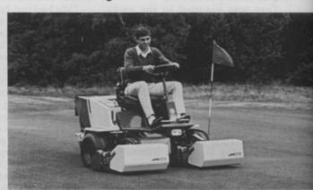
Ransomes has introduced its first all-hydraulic triplex greensmower. The new Greens Triple (above) is out this spring.
