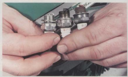
Check spark plugs regularly because a worn spark plug will rob the engine of power.
