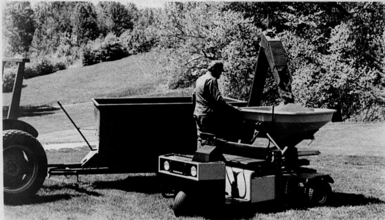
The grain cart auger fills the Vicon Spreader hopper in a matter of minutes at Hercules Country Club.
