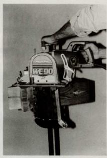
Safety features include a full upper blade guard, a non-removable tip guard and rear pivoting blade guard.
