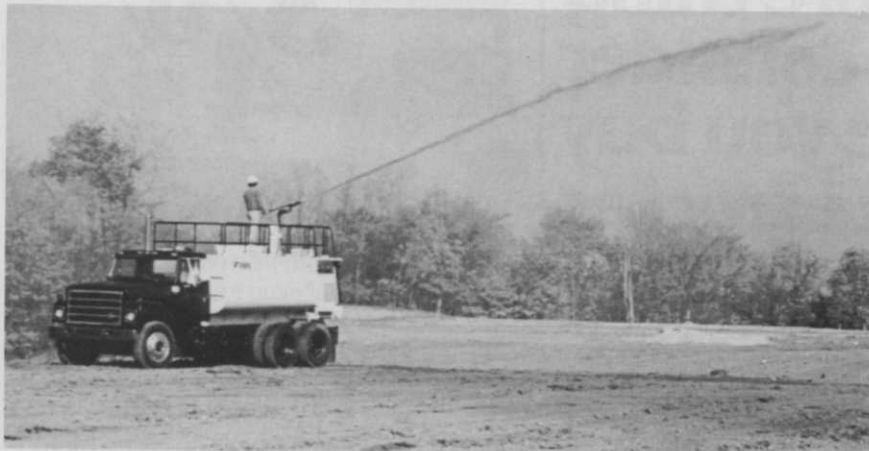
The Finn Corporation's HydroSeeder.
