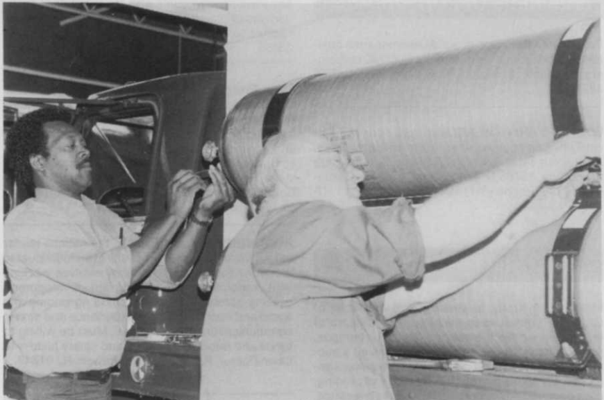
Tanks for storing natural gas are installed as a part of the conversion to dual fuel operation by participants in a seminar on natural gas conversion at Hocking Technical College in Nelsonville, Ohio.
