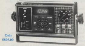
The MT3000 pays for itself many times over by eliminating costly over and under applying of herbicides, pesticides and liquid fertilizer. Simply select your desired rate of chemical application and the MT3000 will maintain that rate regardless of speed or boom control change. Take the guess work and waste from your spray program and watch the savings go in your pocket.
