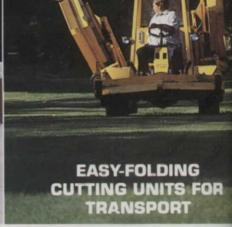
Your search for a high capacity mower encompassing a one man operation is now concluded. The Hydro-Power 180 with its 15 foot hydraulically driven rotary mower has a mowing capacity of up to 11 acres an hour while incorporating rear wheel steering for maximum maneuverability. Cutting units are designed for maximum floatation and may be used individually or in any combination of the three.
