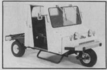
rugged four-cylinder, 40 hp engine. The vehicle can be fitted with pick-up bed, storage box, dumping refuse or turf beds.
