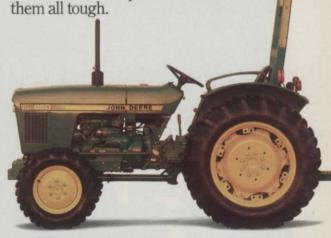
They've all got heavy-duty diesel engines and rugged sliding-gear transmissions. To keep them going strong year after year. They've also got differential lock and optional mechanical front-wheel drive to make the going easier on slopes, banks and other inconvenient places where grass thrives but tractors often fail.
