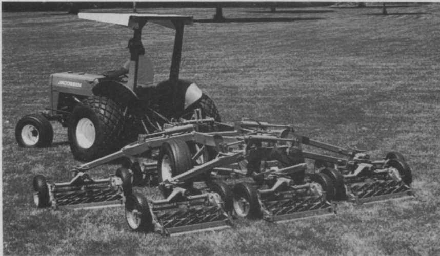
Pull-behind reel gang mowers, like the Jacobsen 5/7 Ram-Lift Ranger with seven gangs, are the most economical mowers for large turf areas.
