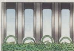
Exclusive roller design features bevelled edges to "pucker-up" horizontal runners.
