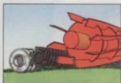
The horizontal reel follows closely behind to clip grass while it's standing straight, for faster, truer greens without lowering height of cut.
