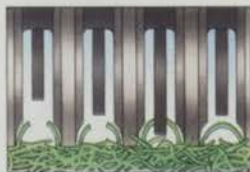
The knife blades rotate through slots in the front rollers, slicing horizontal runners before they lie down.
