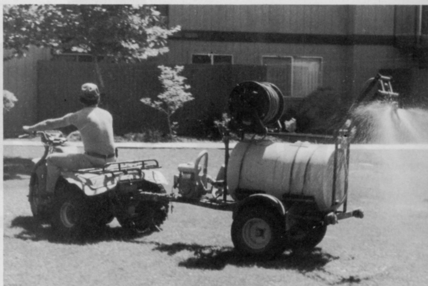
The Tagalong sprayer, designed by Ayers and Baty, is used for fertilizer application on garden apartment turf.
