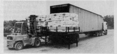
docks. The heavy steel dock is then put into place by a fork lift. When the goods are unloaded from the truck, they can then be transported via pallet, and when empty the dock can be returned to its storage area.
