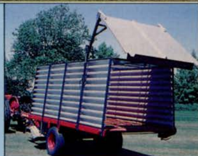
Self unloading with Hydraulic Door
