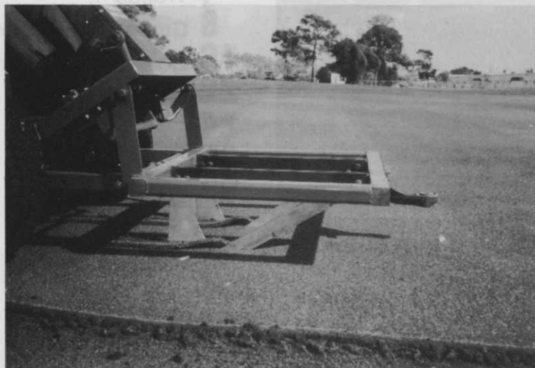
Mascaro's Second Aerifier makes slits instead of holes and has no moving parts.
