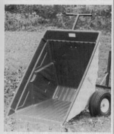
The cart can be operated by hand or can be attached with a tow bar to a farm tractor, lawn tractor or threeor-four-wheeler. It can be dumped with an unloading handle which is easily reached from most tractor seats.
