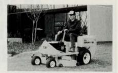
Like the rest of the Hustler product line, the 250 has dual hydrostatic drive for infinite control of speed and power for each drive wheel-forward and reverse. The direct drive wheel motor eliminates chains, sprockets and other high maintenance items that are subject to failure on other
