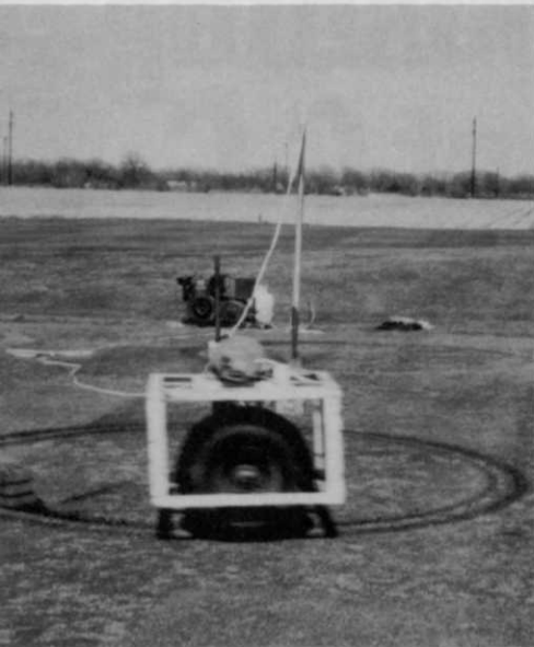
Wear simulator being used to screen wear tolerance. (Photo courtesy of Dr. Jim Beard, Texas A&M)
