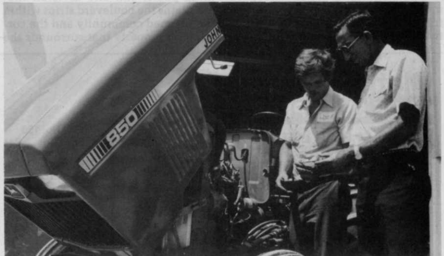
Wayne Poe monitors hours of equipment use to be sure that crankcase oil is changed every 100 hours on a tractor, every 50 hours on a push mower. Carl Smith checks the oil.
