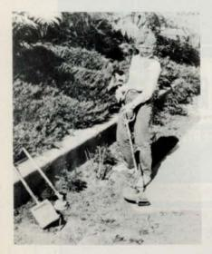
with its adjustable, tilted handle, offers the operator greater reach and comfort without stooping or causing other body strain.
