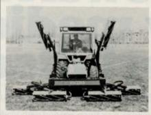
mowers. Additional attachments include side mounted flail cutters, forklift, bucket, sweeper, dozer blade and snow blower.
