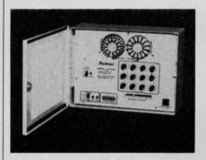
The DD controllers also have the "Time Multiplier Switch" for seasonal adjustment. With 50, 100, and 200 percent settings, the time per station can be cut in half, remain the same, or doubled. LED indicators show which station is operating. The M-12DD and M-24DD have a combination solid-state and electro-mechanical components, and come
