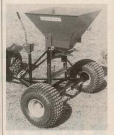
sions of the trailer are 60 in. wide and 60 in. long. It comes complete with two high flotation tires, clevis hitch, and battery box (battery not included). The seeder's 12-volt motor can also be wired into the vehicle's electrical system.
