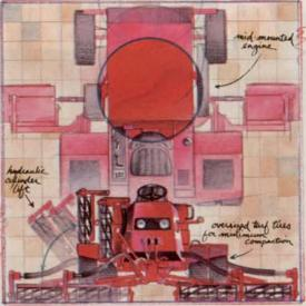
hydraulic cylinder lift raises the two outside mowers in a few seconds. So you can quickly narrow your cutting path around trees, traps, fences, flower beds, and other obstacles. Without slowing your pace.
