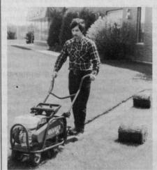
thickness of cut is quick and easy to adjust with the Mark 2. The sod cutter comes equipped with a 5-hp engine. **Circle No. 190 on Reader Inquiry Card**
