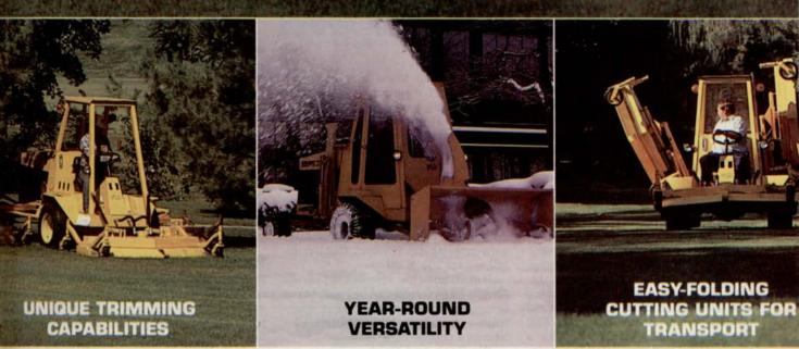
Your search for a high capacity mower encompassing a one man operation is now concluded. The Hydro-Power 180 with its 15 foot hydraulically driven rotary mower has a mowing capacity of up to 11 acres an hour while incorporating rear wheel steering for maximum maneuverability. Cutting units are designed for maximum floatation and may be used individually or in any combination of the three.
