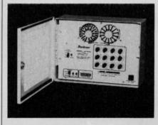
The DD controllers also have the "Time Multiplier Switch" for seasonal adjustment. With 50, 100, and 200 percent settings, the time per station can be cut in half, remain the same, or doubled. LED indicators show which station is operating. The M-12DD and M-24DD have a combination solid-state and electro-mechanical components, and come standard with lightning protection on the input and each output of the valves.
