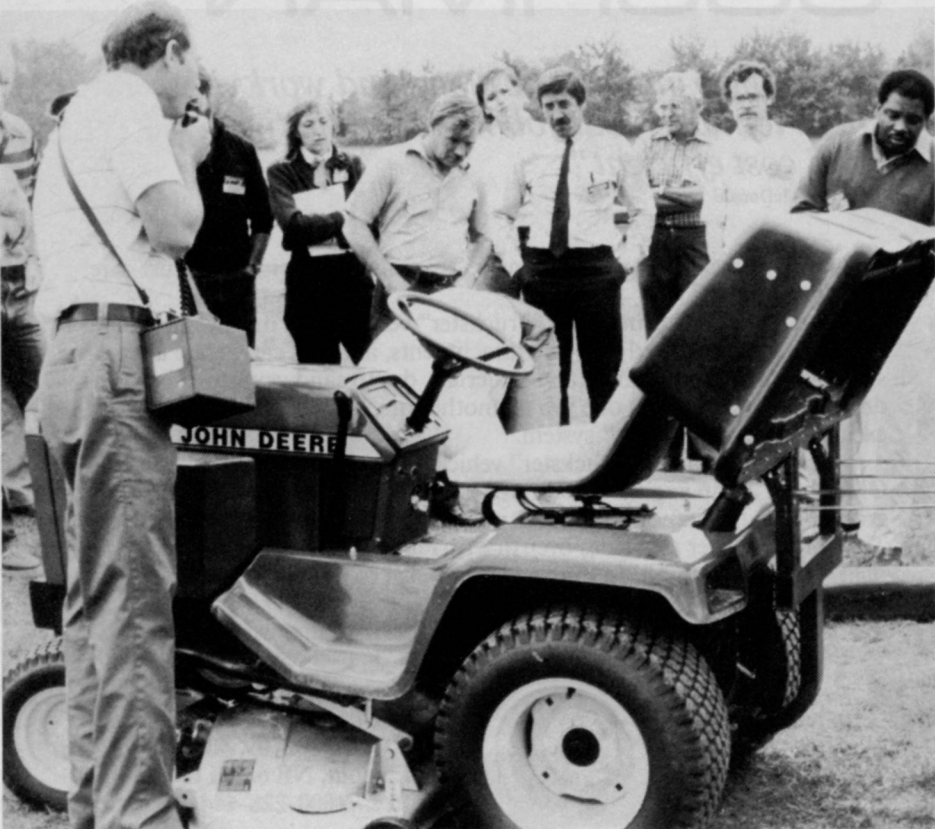
John Deere personnel attach the Power Flow bagging system to a lawn tractor.
