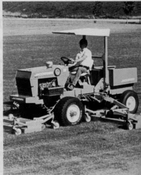
Jacobsen's HR-15 can cut 16-foot swath
