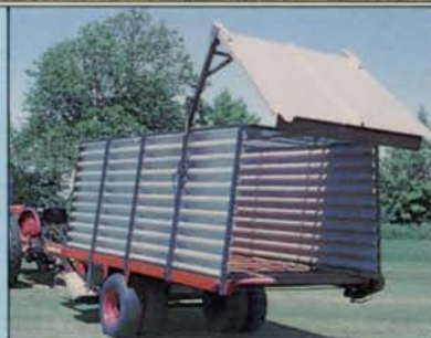
Self unloading with Hydraulic Door
